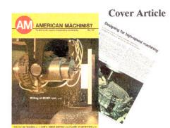
"That machine, designed specially for display at the International Machine Tool Show in Chicago . . . attracted a fair amount of attention for its builder, Turchan Inc (Dearborn, Mich), because of its use of a 20-hp, 60,000-rpm magnetically levitated spindle, the first time such a spindle had ever been displayed milling metal."
